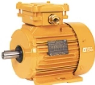
– 3-phase TEFV induction motors, **FLSPX series with cast iron housing**, conforming to IEC 34, 72, EN 50281, power **0.18 to 400 kW**, frame size 80 to 355 mm.
