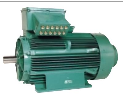
– 3-phase TEFV induction motors, FLS series with cast iron housing, conforming to IEC 34, 72, EN 50281, power 0.18 to 750 kW, frame size 80 to 450 mm.
